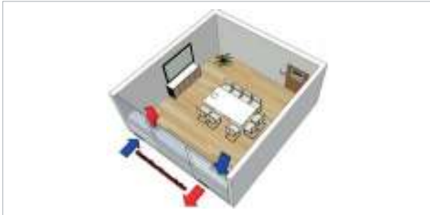
Each master unit is connected to a maximum of one slave unit.
