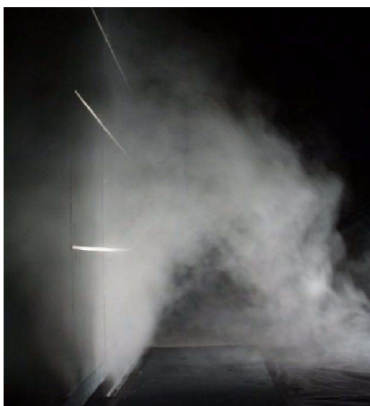
Picture 2: Visualization of indoor air flow, 45 m³/h and -6 K
