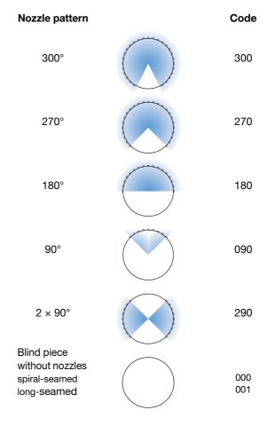
The blind piece is a specially made spiral-seamed pipe that resembles ventiduct in design, as it has no actual nozzles.
