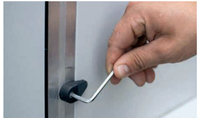
Figure 22: The overpressure doors and de-mounting service covers are attached to the housing by blockers. To remove / attach the blockers use a 4 mm imbus key.
