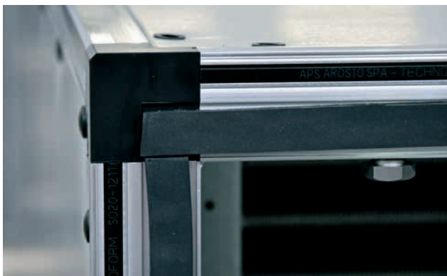
Figure 15: The sealing tape must overlap at the corners. When connecting two sections, apply the sealing tape only on one of the sections.
