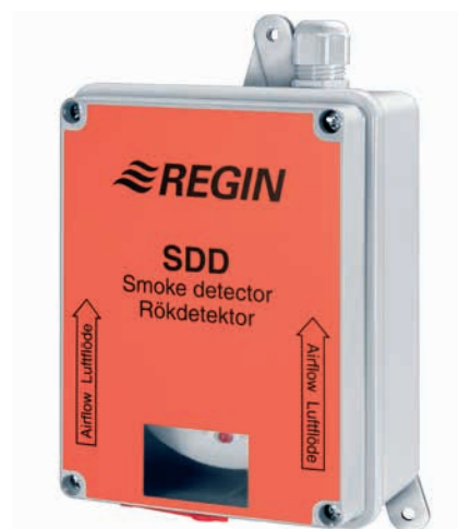
Figure 56: Smoke detector. Works on optical detection and has a built-in relay for alarming. When the smoke detector is activated, the unit stops as in case of fire.
