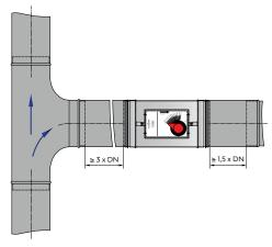
The specified control accuracy of  $\Delta \dot{V}$  can only be achieved with at least 3 x DN straight flow path.
